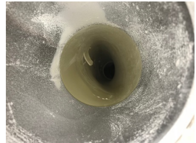
Deteriorated Hose Interior
