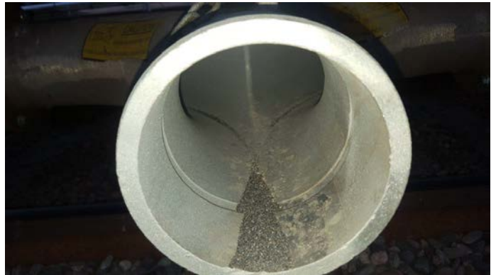
Metal filings in product line after wash. Vessel should be rejected back to shop for cleaning, additional wash followed by a product flush.
