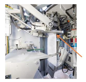
Positioning of the filled bag on the transport belt
