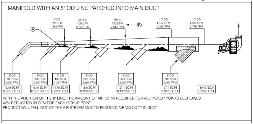
Dust is NOT in suspension; System is NOT balanced. Air taking path of least resistance.
