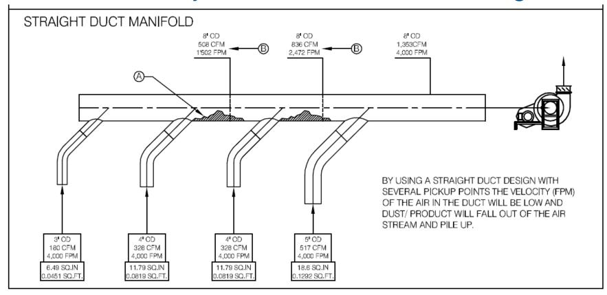
Dust is dropping out (in locations); System is balanced (at end of system).
