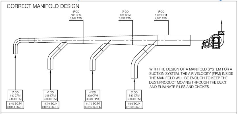
Dust is in suspension; System is balanced.
