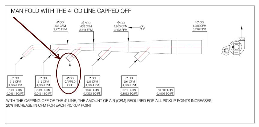
20% increase in CFM at each pickup point. May not be an issue, but will increase velocity and may pick up good product (i.e. good grain going to feed).
