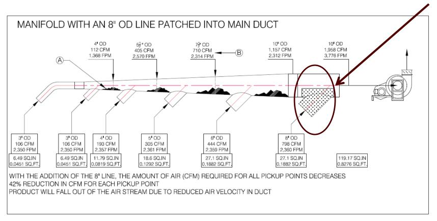
42% reduction in CFM at each pickup point and allows product to drop out of the line
