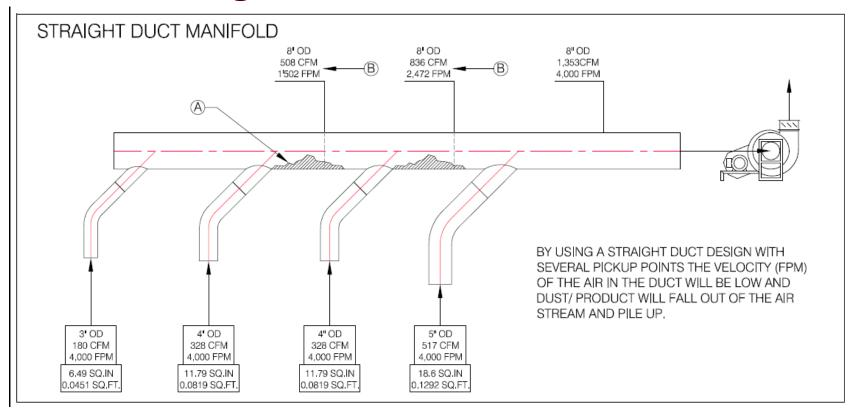
Easier, simpler, and less expensive to install but allows for several points along the line for product to drop out due to velocity.
