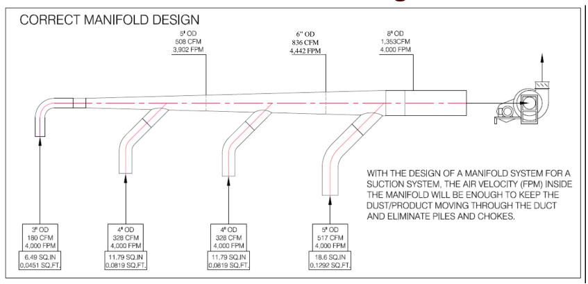
Designed to keep air velocity inside the duct high enough to keep product moving and eliminate product laying in the line
