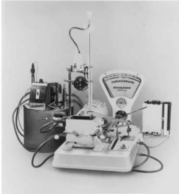
1928: The First Farinograph® World's first wheat and wheat flour quality tester
