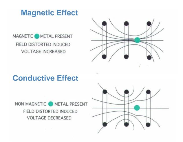
In the APEX Magnetic = X and Conductive = R
