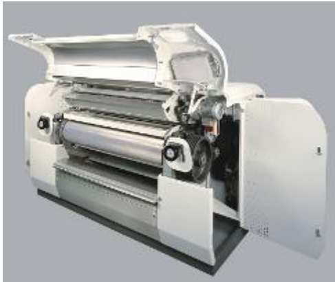
Easy access for cleaning Example MDDR Roller Mill
